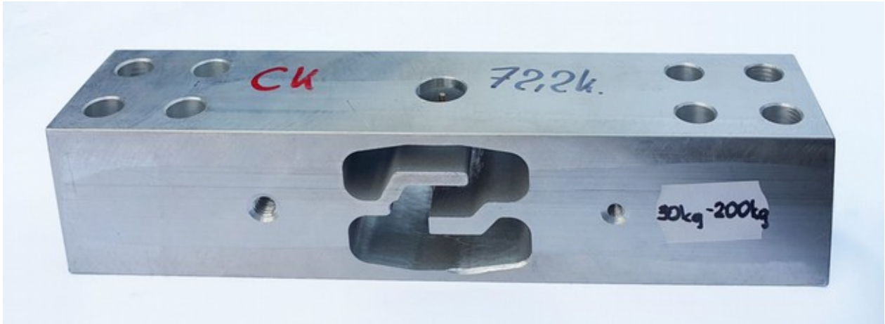
Fig.3 Measuring beam with variable cross-section of measuring springs
